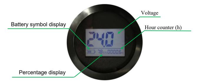
The unit of the hour counter is in hours, and the minimum resolution is 0.1h (6 minutes). The symbol "h" flashes at the frequency of 1 Hz.
